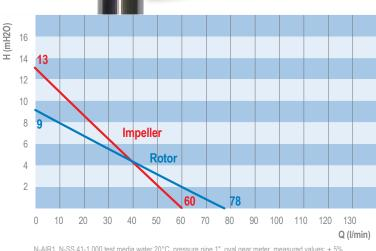
N-AIR1, N-SS 41-1,000 test media water 20°C, pressure pipe 1", oval gear meter, measured values: ± 5%
